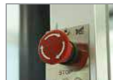
Emergency Stop Button
