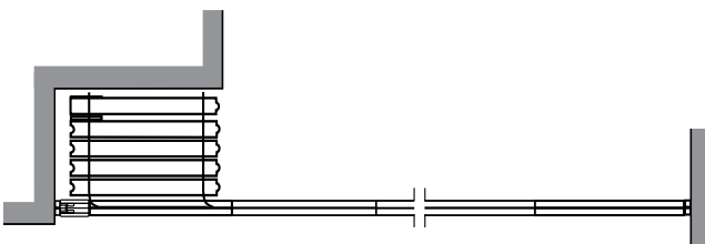
Two Point Suspension & parallel to track
